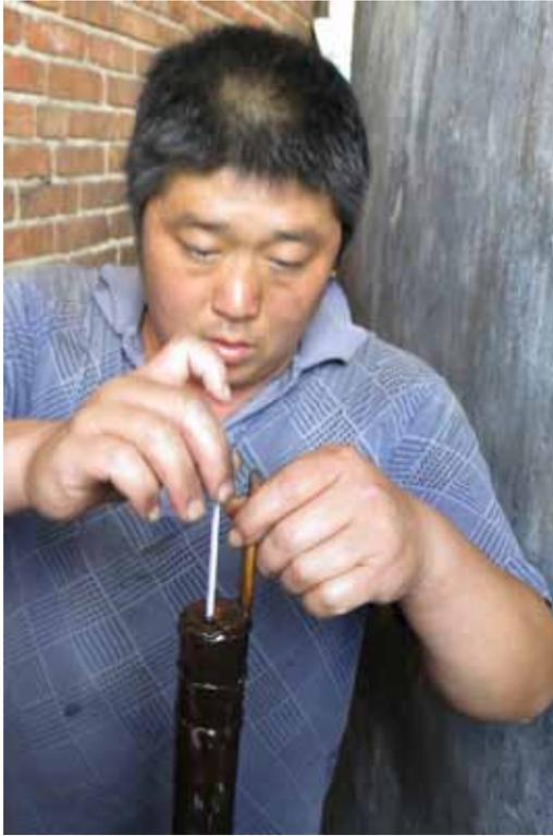
Testing alcohol for ABV with hydrometer.
