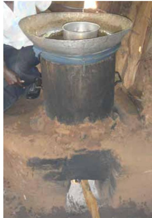
Complete setup of the distillation process for *changa* production.
